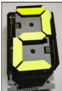
bistabile Klappanker- ziffer
